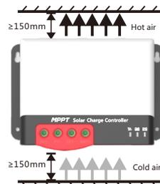
Figure 2.1 Installation and Heat Dissipation
